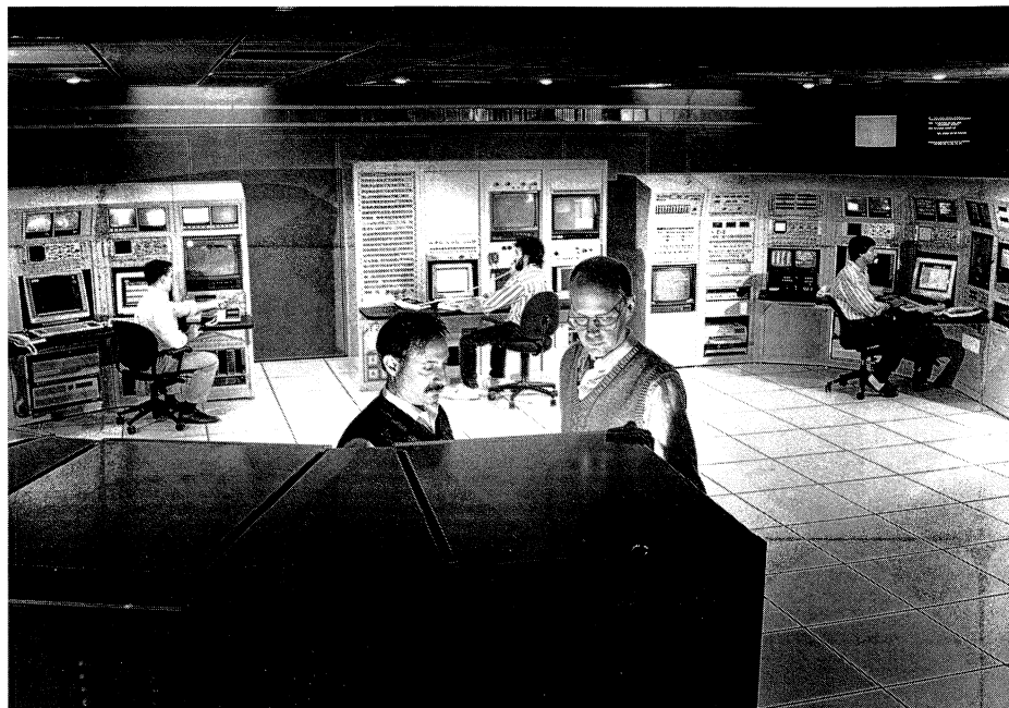
The control room for Brookhaven's AGS synchrotron has been remodelled and expanded to cover all linked machines (Linac, Booster). It features five general purpose consoles based on networked Apollo workstations, plus a special safety console (centre rear). In the foreground are AGS operations head Peter Ingrassia (left), and AGS controls section head Don Barton.
